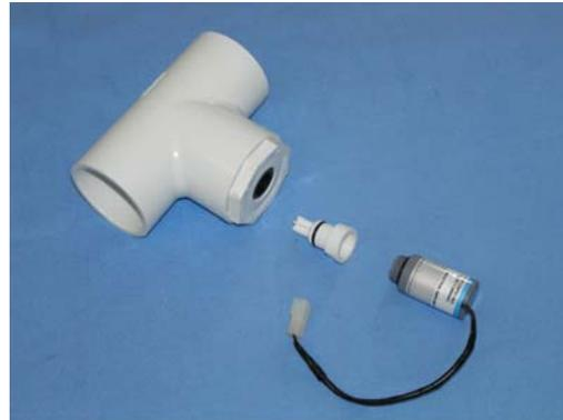
Note: If your mixing stick is built from something other than 1-1/2 inch PVC, you can purchase the correct size “T” at your local hardware store. Make sure that the part where the oxygen sensor goes has a 1/2” pipe thread. Remove the black sleeve from the provided 1-1/2” PVC “T” with your fingers. Do not use tools as you will mar the inside surface and the oxygen sensor/diverter will not fit or seal properly.
